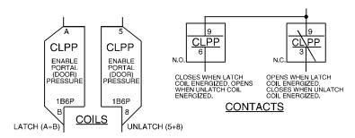
**CL=Control, Latch Relay** A relay which latches in an energized or set position when operated by one coil (the *latch/set coil*). The relay stays latched, even though coil voltage is removed. The relay releases or unlatches when voltage is applied to a second coil, (the *unlatch/reset coil*).
