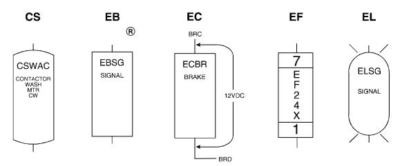
**CS=Control, Contactor/Motor Starter** A relay capable of handling heavier electrical loads, usually a motor.
