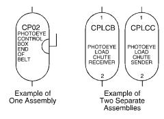
**CP=Control, Photo-Eyes** Photo-eyes sense the presence of an object without direct physical contact. Photo-eyes consist of a *transmitter, receiver, and output module*. These components may be housed in one assembly with the transmitter bouncing light off of a reflector to the receiver, or these components can be housed in *two separate assemblies* with the transmitter pointed directly at the receiver.
