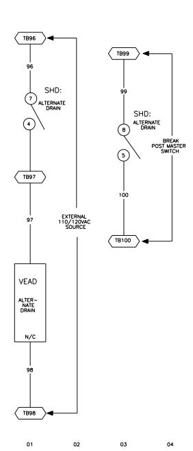
W6V5WSDR SCHEMATIC: ALTERNATE DRAIN VALVE FOR AIR OPERATED DRAINS ONLY 110V1P50HZ/120V1P60HZ
