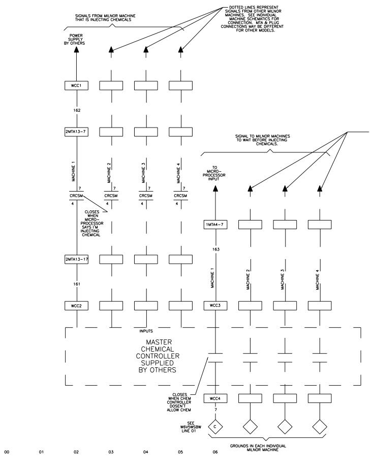
DOTTED LINES REPRESENT SIGNALS TO OTHER MILNOR MACHINES SEE INDIVIDUAL MACHINE SCHEMATICS FOR CONNECTION. MTA & PLUG CONNECTIONS MAY BE DIFFERENT FOR OTHER MODELS.
