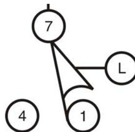
**SM=Switch, Mechanically Operated (Figure 15)**—A switch that is mechanically operated by a part of or the motion of the machine (e.g., door closed switch, tilt limit switches, etc.)
