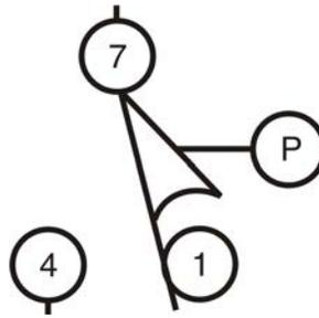
**ST=Switch, Temperature Operated (Figure 17)**—A switch that is actuated at a preset temperature (e.g., dryer safety probes) or has adjustable set points (e.g., Motometers or Combistats).
