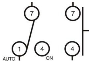
**SK=Switch, Key Lock (Figure 13)**—A switch that requires a key to operate. This prevents unauthorized personnel from gaining access to certain functions (e.g., the *Program menu*).
