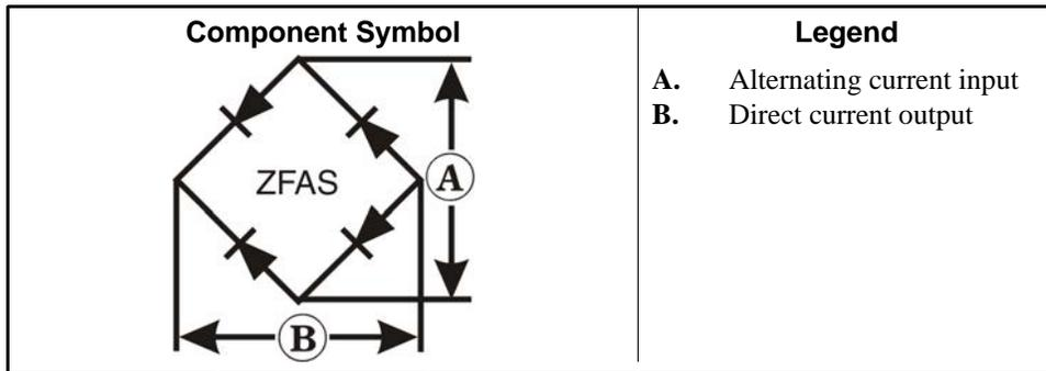
Figure 21: Bridge Rectifier
