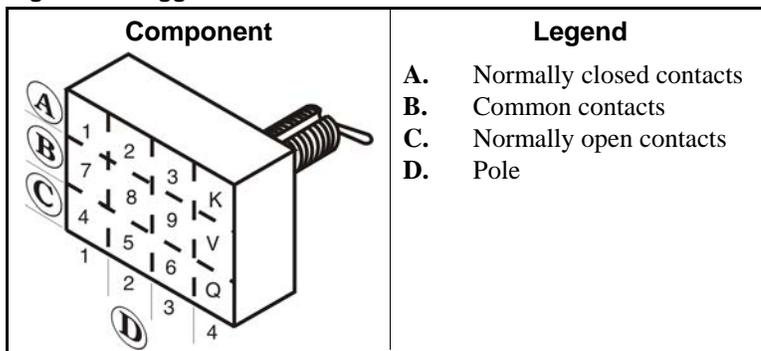
Figure 27: Switch with Replaceable Contact Blocks
