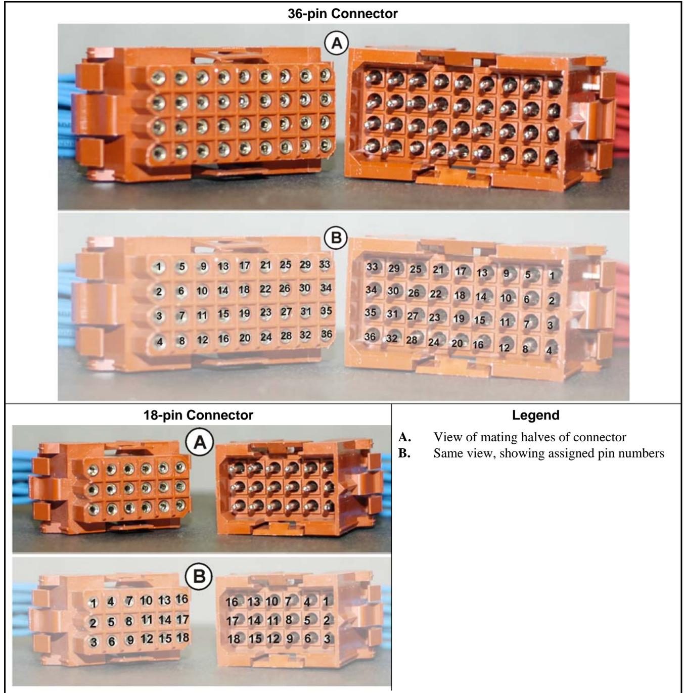
Figure 24: Molex Connector Pin Locations
