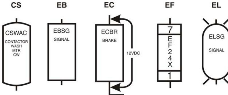
**EB=Electric Buzzer (Figure 6)**—An audible signaling device.
