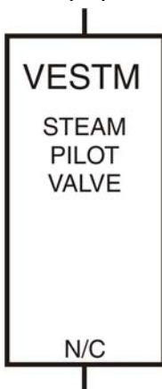
Figure 19: Electrically Operated Valve (VE)
