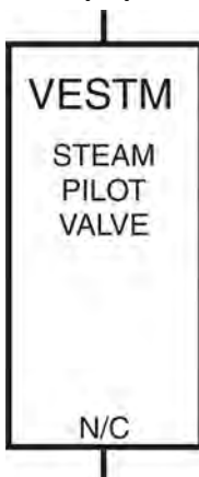
Figure 19: Electrically Operated Valve (VE)
