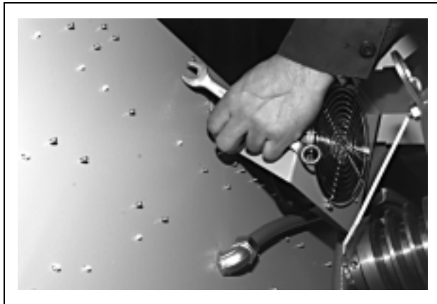
FIGURE 7 (MSSM0285AE) Removing Fan For Hoist Clearance
