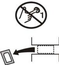
B2T2002013: Do not start the machine until shipping restraints are removed. This tag will appear on the outside of the machine to alert you to the presence of internal shipping restraints. A tag will also appear on the restraint to help identify it. Most, but not all shipping restraints display the color red. Some shipping restraints are also safety stands. Do not discard these.
