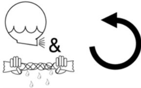
B2TAG94097: The cylinder must rotate **counterclockwise** during draining and extraction (spin) when viewed from here (rear of machine). Otherwise, reverse the electric power connections, as explained in the schematic manual.
