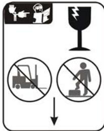
B2TAG94078: Do not forklift here; do not jack here; do not step here—whichever applies.
