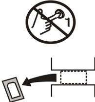
B2T2002013: Do not start the machine until shipping restraints are removed. This tag will appear on the outside of the machine to alert you to the presence of internal shipping restraints. A tag will also appear on the restraint to help identify it. Most, but not all shipping restraints display the color red. Some shipping restraints are also safety stands. Do not discard these.
