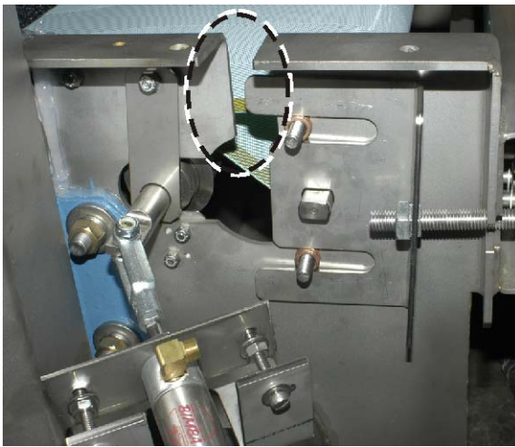
Figure 26: Tank Left Side Wall With Slot
