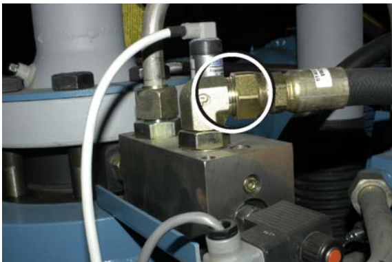
Figure 52: Bypass Valve: Where to Disconnect Hose
