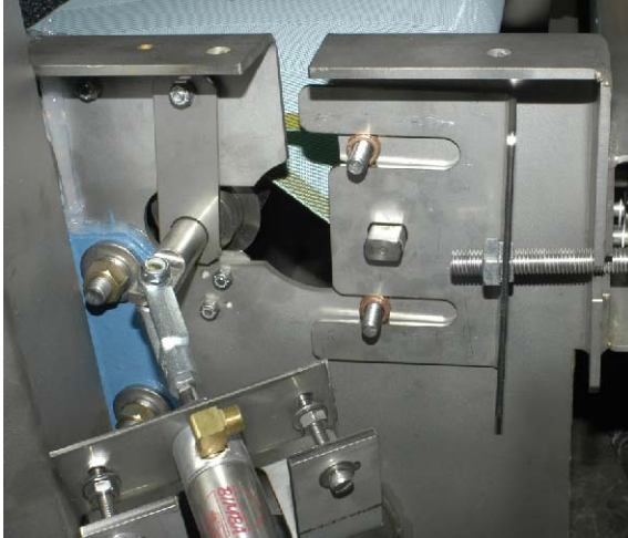
Figure 29: Tracking Bracket and Related Components Hanging from Tracking Roller
