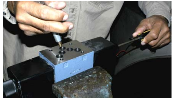
Figure 50: Bench-testing a Directional Valve
