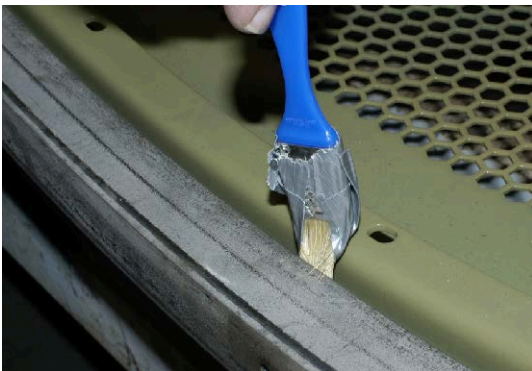
Figure 27. Adhesive applicator—1" paint brush, bristles held at an angle with tape
