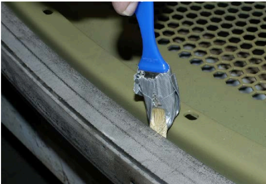
Figure 16. Adhesive applicator—1" paint brush, bristles held at an angle with tape
