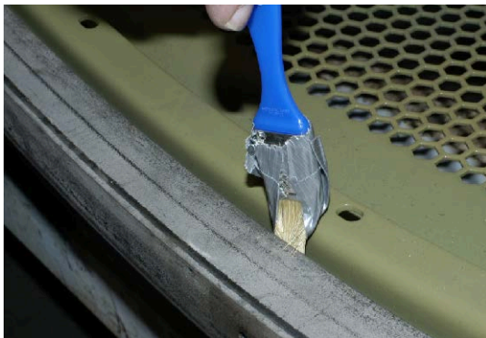
Figure 11. Adhesive applicator—1" paint brush, bristles held at an angle with tape
