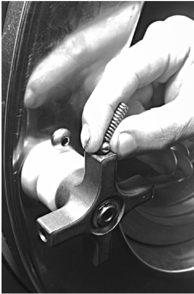
Figure 19. Inserting Ball and Spring in Handle Spoke
