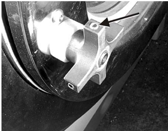
Figure 10. Door Handle Spoke Set Screw
