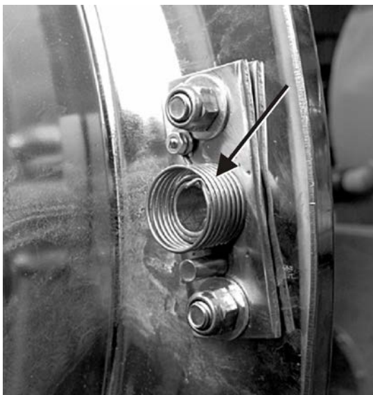
Figure 14. Return Spring After Separation from Shaft Cam
