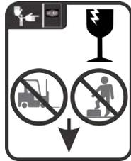
B2TAG94078: Do not forklift here; do not jack here; do not step here—whichever applies. (Not used on MCT models.)
