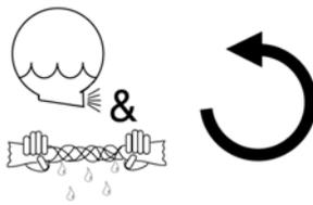
B2TAG94097: The cylinder must rotate **counterclockwise** during draining and extraction (spin) when viewed from here (rear of machine). Otherwise, reverse the electric power connections, as explained in the schematic manual.
