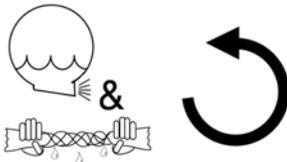
B2TAG94097: The cylinder must rotate **counterclockwise** during draining and extraction (spin) when viewed from here (rear of machine). Otherwise, reverse the electric power connections, as explained in the schematic manual.
