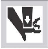
**WARNING: Entangle and Crush Hazards** — Contact with moving components normally isolated by guards, covers, and panels, can entangle and crush your limbs. These components move automatically.
