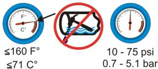
B2T2008007: Do not exceed 160° Fahrenheit (71° Celsius) water temperature. Excessive temperature can damage the water valves in this machine. Eliminate water hammer on the water lines to this machine. Water hammer can rupture the water inlet valves on this machine. Follow applicable codes when installing water hammer arresters. Maintain incoming water pressure between 10 and 75 psi (between 0.7 and 5.1 bar). Pressures outside this range can damage the water valves in this machine.
