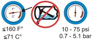
B2T2008007: Do not exceed 160° Fahrenheit (71° Celsius) water temperature. Excessive temperature can damage the water valves in this machine. Eliminate water hammer on the water lines to this machine. Water hammer can rupture the water inlet valves on this machine. Follow applicable codes when installing water hammer arresters. Maintain incoming water pressure between 10 and 75 psi (between 0.7 and 5.1 bar). Pressures outside this range can damage the water valves in this machine.
