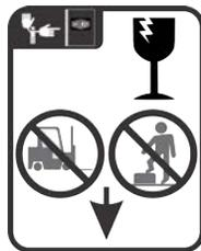
B2TAG94078: Do not forklift here; do not jack here; do not step here—whichever applies. (Not used on MWT models.)
