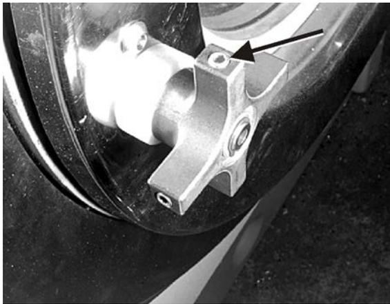
**Figure 11. Handle Spoke Spring and Ball**
