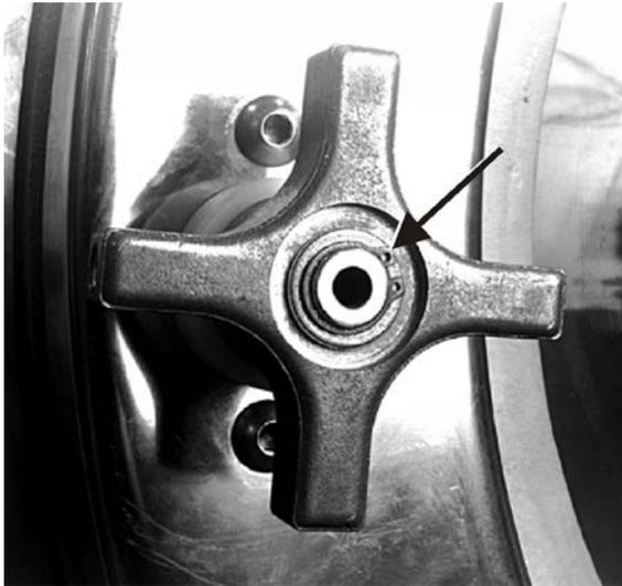
**Figure 13. Rear Flange Bearing (being removed) and Retaining Clip (arrow)**
