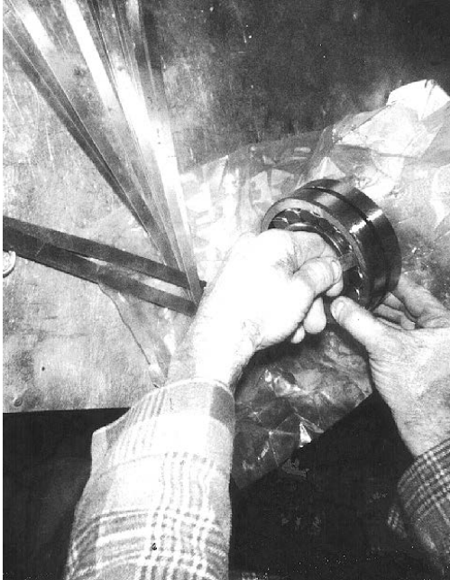
Figure 38. Measuring Bearing Unmounted Clearance (bridge for 42" machine shown)
