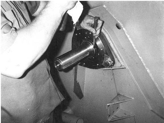
Figure 39. Tightening the Bearing Lock nut (42" machine shown)
