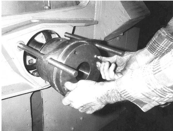
Figure 35. Installing the Bearing Housing Setting Fixture onto Housing (42" machine shown)
