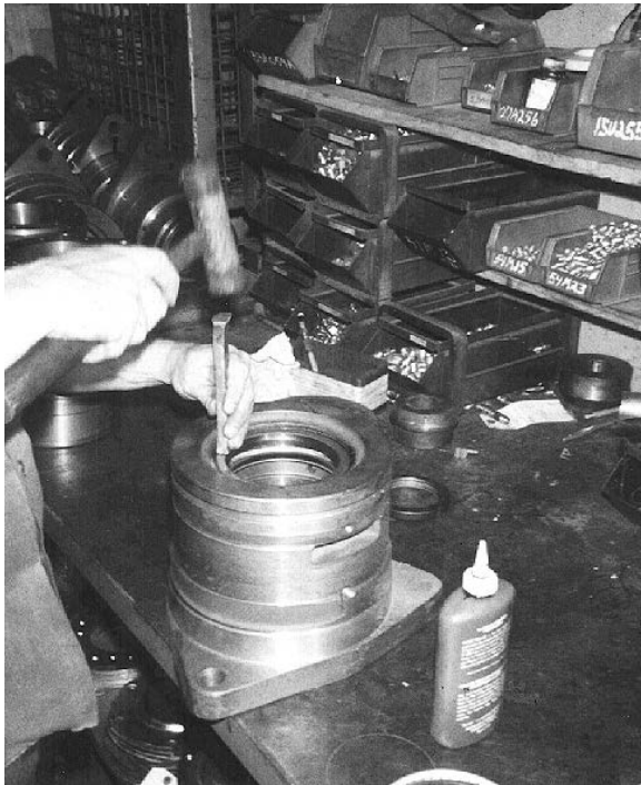
Figure 33. Installing Seals in Bearing Housing
