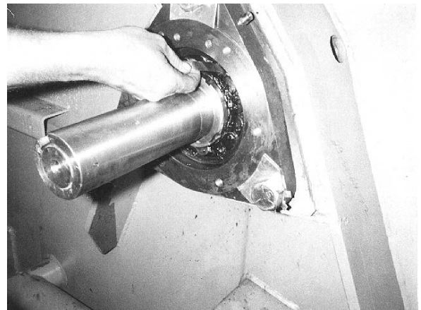
Figure 36. Measuring the Mounted Internal Clearance of the Bearing (42" machine shown)
