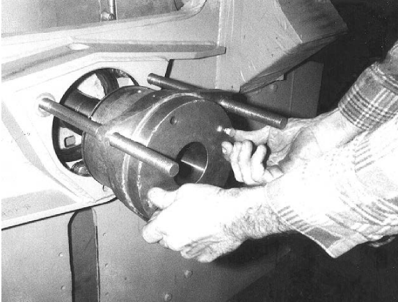
Figure 31. Installing the Bearing Housing Setting Fixture onto Housing (42" machine shown)
