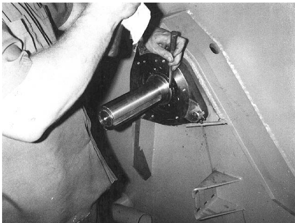
Figure 35. Tightening the Bearing Lock nut (42" machine shown)
