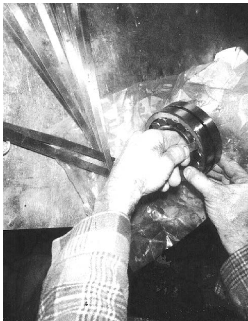
Figure 34. Measuring Bearing Unmounted Clearance (bridge for 42" machine shown)
