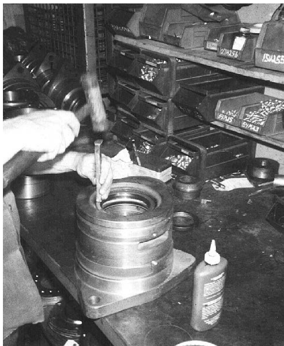
Figure 29. Installing Seals in Bearing Housing
