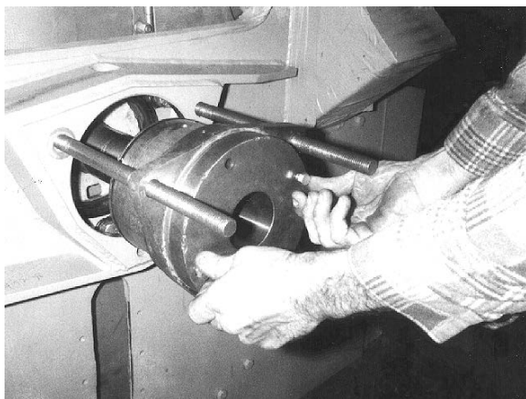
Figure 34. Installing the Bearing Housing Setting Fixture onto Housing (42" machine shown)
