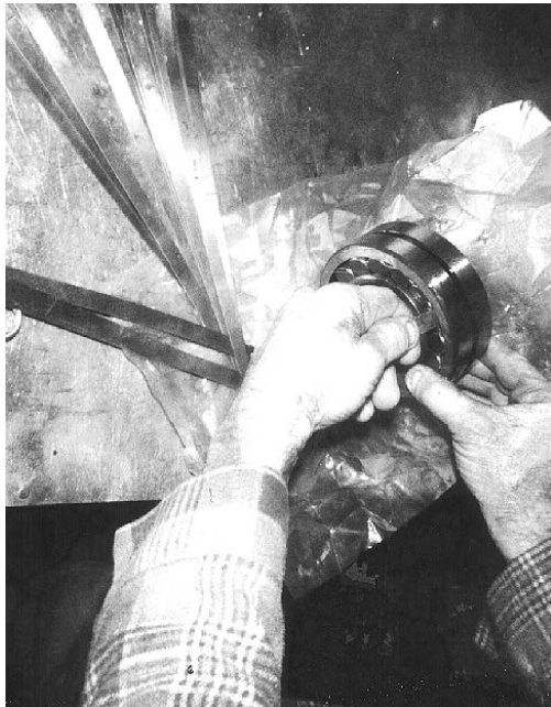
Figure 37. Measuring Bearing Unmounted Clearance (bridge for 42" machine shown)
