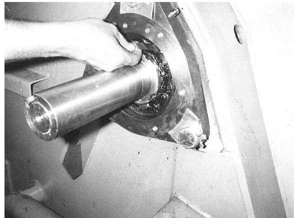
Figure 39. Measuring the Mounted Internal Clearance of the Bearing (42" machine shown)
