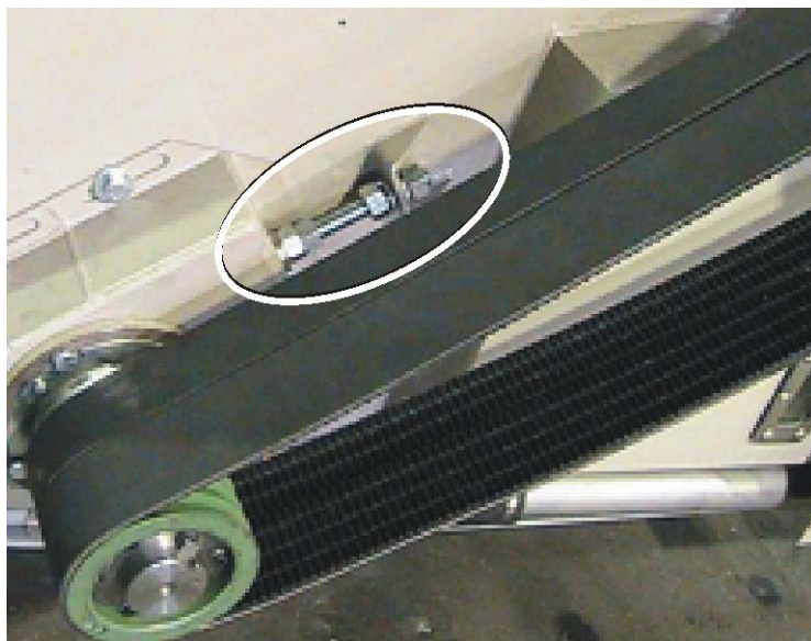
Figure 23. Some Pairs of Tension Mechanisms that Can Change the Angle of the Pulleys
