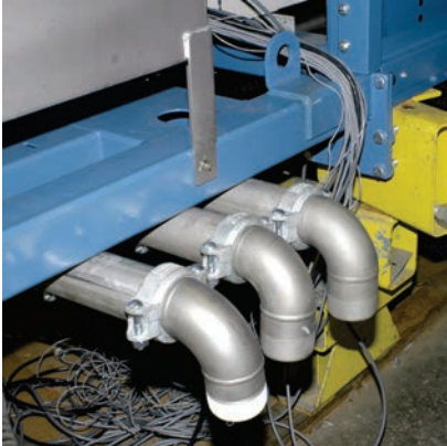
Water Inlets (One fresh water inlet to tank is standard; maximum is four.)
