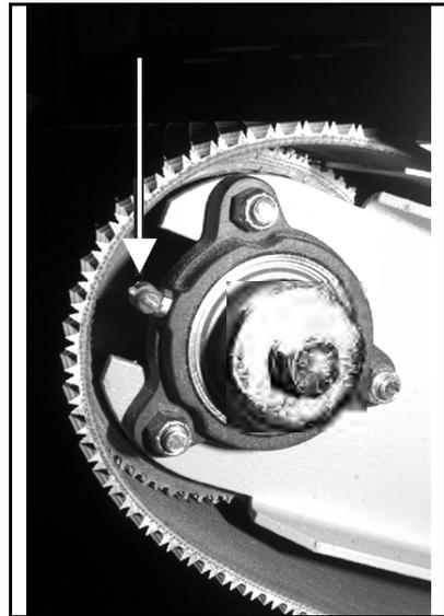
Figure 7: Conlo and Conwa brake adjustment
