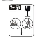
B2TAG94078: Do not forklift here; do not jack here; do not step here—whichever applies.
