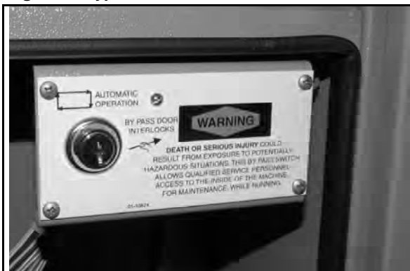
Figure 1: Bypass door switch
