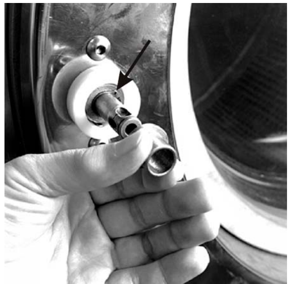
Figure 4: Rear Flange Bearing (being removed) and Retaining Clip (arrow)
