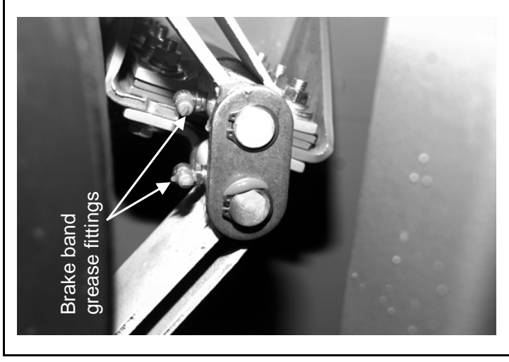
FIGURE 22 (MSSM0201CE) Brake Band Grease Fittings (60044 and 72044WP2/WP3)
