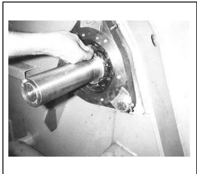
FIGURE 12 (MSSM0303AE) Measuring the Mounted Internal Clearance of the Bearing (42" machine shown)
