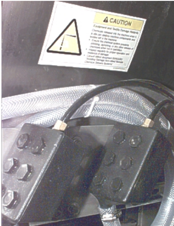
Figure 1: Pumped Chemical Inlets on CBW Batch Washer
