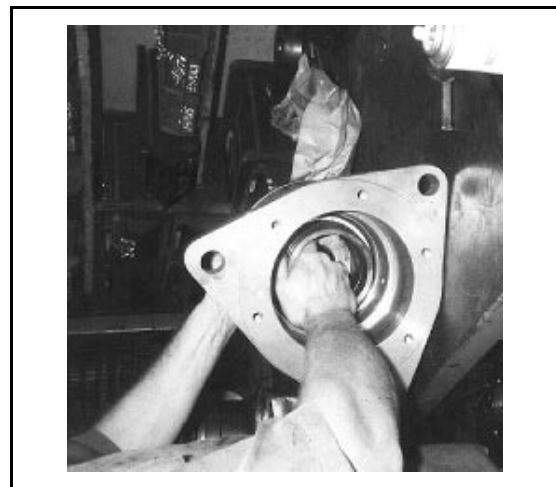
FIGURE 6 (MSSM0303AE) Installing Seal Sleeve in Bearing Housing
