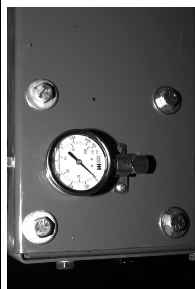
FIGURE 25 (MSSM0201CE) Hydraulic Tilt Pressure Gauge (On rear of 42" , 48" , and 72" tilt models)
