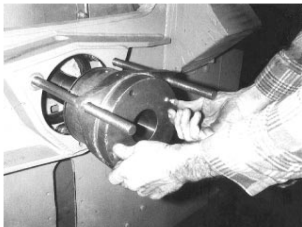
FIGURE 7 (MSSM0303AE) Installing the Bearing Housing Setting Fixture onto Housing (42" machine shown)
