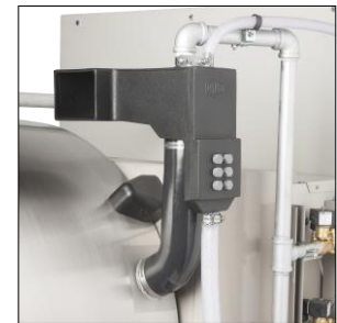
Safe chemical injection
