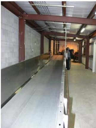
The latest expansion consisted of: a Milnor 4 Compartment CONWA04 Loading/Weighing Conveyor, a four-module 76039 CBW tunnel washer, a 700 RPM M7V4836C high speed centrifugal extractor, two Milnor
