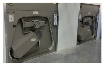
HYGIENIC SEPARATION: A barrier wall runs throughout the plant to ensure separation between soiled and cleaned linen. The plant has two Milnor Staph Guard barrier washers and plans to install two more
