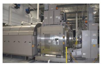
ECO EFFICIENT: The plant is eco efficient and its two Milnor PBW $^{\text{TM}}$  tunnel lines process up to 2,100kg (4,700lb) per hour with an average fresh water consumption of 3.49litres/kg (0.42gallons/lb)
