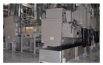
SAFE AND DRY: The dryer pod avoids the need for shuttles and helps to promote safe operation
