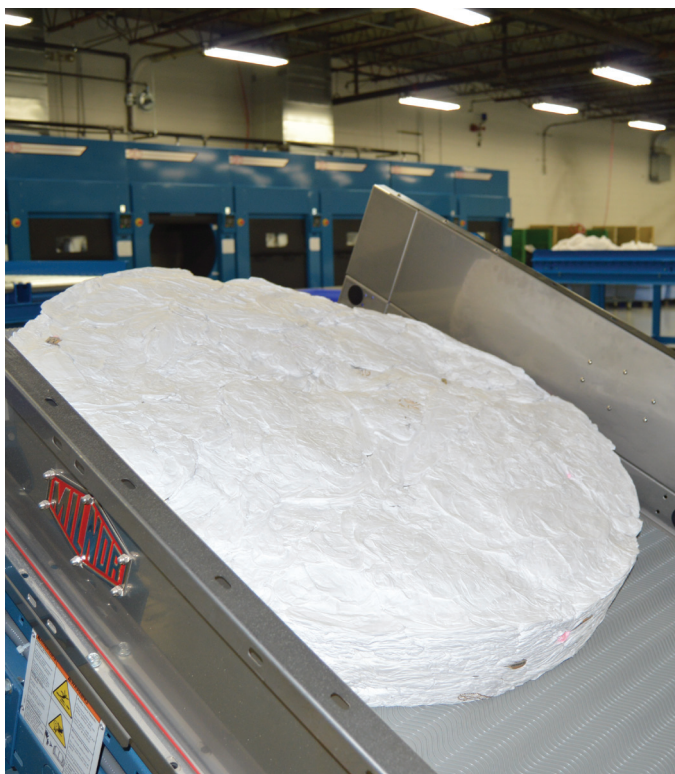
CAKE DELIVERY: Pressed cakes are delivered straight from the 40bar single-stage press to the dryers
