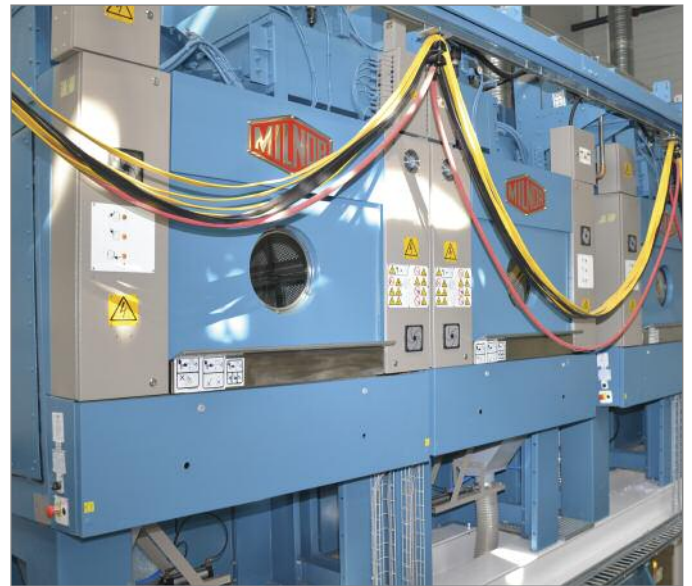
THREE-TIER SOLUTION: To increase production within the original space, Milnor helped to devise a three-tier layout. The dryers are fed by an automated linen elevator and a rail system delivers linen from the dryers to the finishing stations
