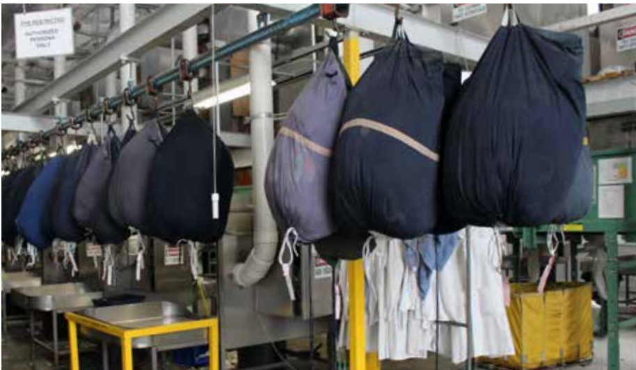
(clockwise from top) A view of the control center for Service Linen Supply's tunnel washer; garments in motion in the plant; bags of soiled linen move to the soil-sorting area; and garments outfitted with RFID chips pass by RFID tracking equipment.
