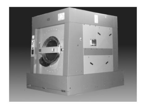
The factory recommends dissassembling the top frame members, perhaps leaving the rear columns with electric box and supply connected. The shell may still be mounted to the bottom frame and also shipping brackets, which may help support the shell until ready to lift it off.
