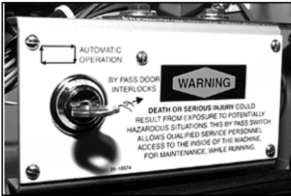
Figure 1: Bypass door interlock key switch
