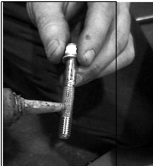
Figure 8: Putting Loctite 242 on diaphragm mounting bolts
