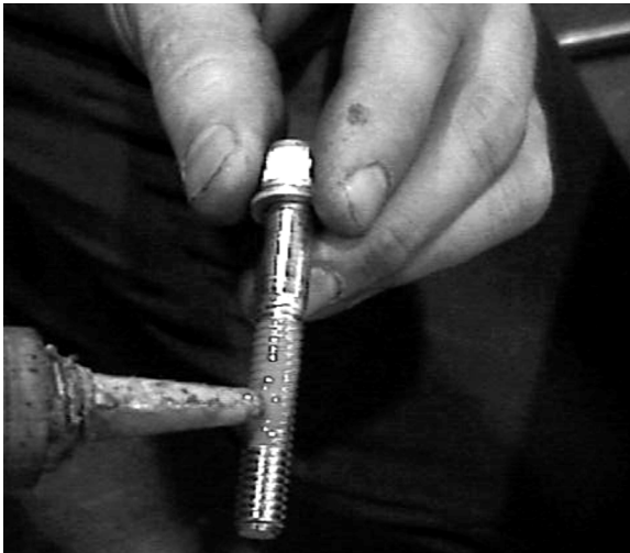
Figure 4: Applying Loctite 242 to Bolts
