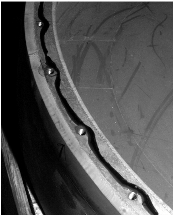
Figure 3: Loctite 515 Applied to Diaphragm Ring
