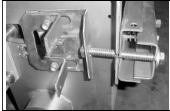
Figure 7: Install belt tension support & bar, hex tap screw & captive nut and air cylinder mounting bracket
