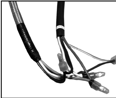
Figure 8: Install motor wiring
