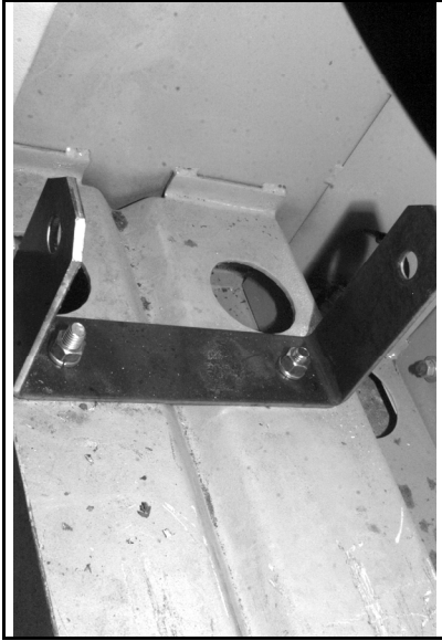
Figure 3: Installed motor bracket (mount tall side towards front of machine)
