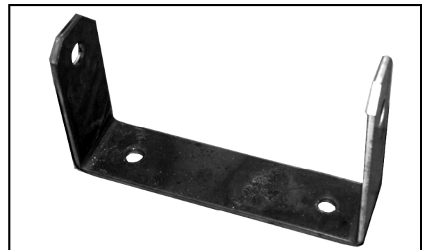
Figure 2: New motor mount bracket (install with tall side to front)
