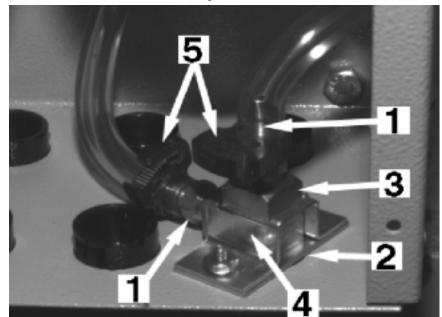
needs to be installed between the pressure transducer and the tee. The other needs to be installed between the pressure switch and the tee. Cut both pieces of tube so that when they are installed there is some slack. Cut the tube at a 90 degree angle. After cutting the tubes, install them using the hose clamps (figure 1, number 6 and figure 2, number 5) supplied.
