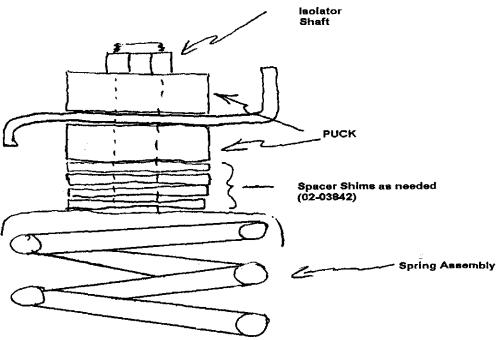
In Step 8 of instructions, the installation of shims should be added.
