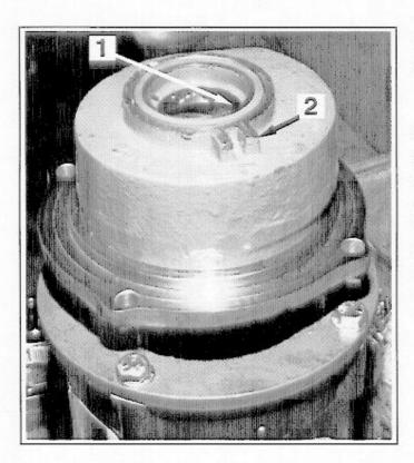
.005" feeler gauge to check the clearance between the diffuser and the impeller. Refer to figure 8, item 1. If the clearance is incorrect, add or remove spacers as needed (drawing 27E958K74 items 10 and 11). Figure 8, item 2 shows the notch on the diffuser that needs to be aligned with the pump housing notch, figure 9, item 1. Install the new pump housing seals. refer to drawing 27E958K74 item 6. Bolt the pump housing to the pump adapter.
