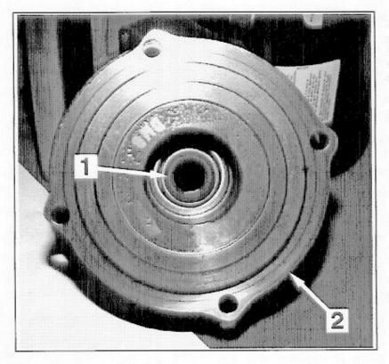
Figure 2 shows the ceramic rotary seal. Item 1 is the seal spacer. Item 2 is the rubber gasketed ceramic mating ring. Item 3 is a cardboard disc placed between the seal halves to protect the seal surfaces during shipment. Discard the cardboard disc before seal installation. Item 4 is the purebide E siliconized graphite seal ring.
