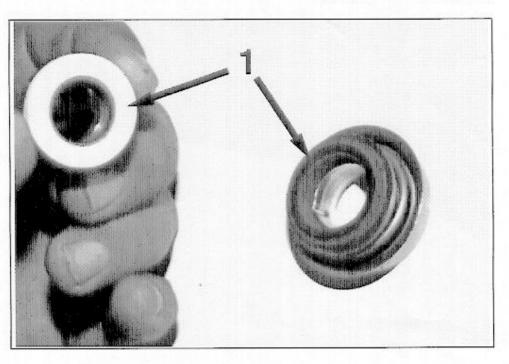
install. It is very important that no grease or any other foreign matter, including finger prints and seal lubricant, get on the mating surface of the seal. Contaminants on these
