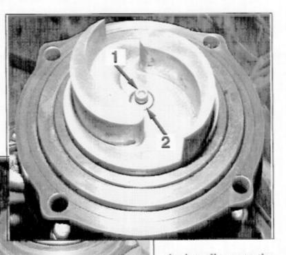
the impeller onto the shaft. Put the spacer in the hole in the impeller. Refer to figure 7, item 2. Thread and tighten the impeller retainer
