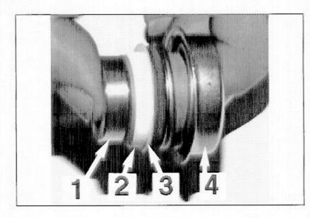
surfaces will cause the seal to fail prematurely. Figure 1 item 1, shows the ceramic rotary seal's mating surfaces.
