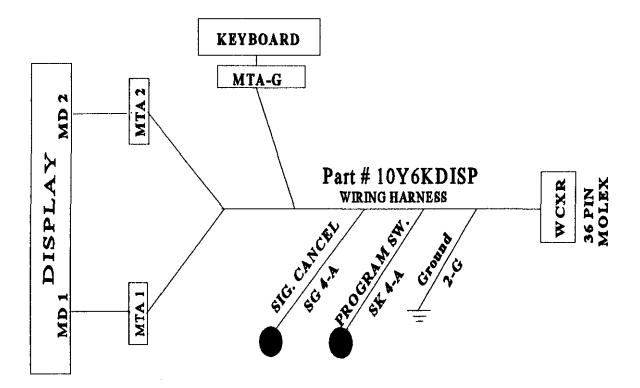
This Harness is supplied with the kit and replaces the 36 pin Molex connector WCXP currently connected to the display, key board and switches.
