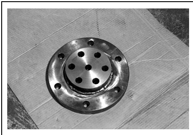
FIGURE 5 (MSSM0275AE) Shaft Cap Fixture Showing Raised Surface
