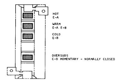
NOTE: HOT, WARM AND COLD SWITCHES INTERLOCK AND REMAIN DEPRESSED.
