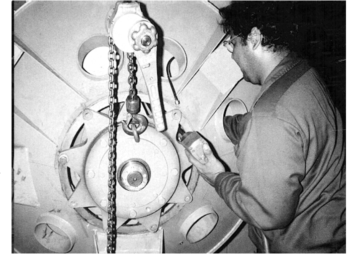
FIGURE 7 (MSSMA403AE) Unbolting the Bearing Housing
