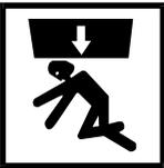
**CRUSH HAZARD**—Descending main bell will crush anyone under it. Bell can descend even with power off.
