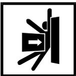
**COLLISION, CRUSHING, AND PINCH HAZARDS**—Serious bodily injury or death can result to personnel in proximity to machinery/systems that traverse, elevate, extend, pivot, and/or tilt. The following mandatory minimum safety requirements must be installed with the machinery system:
