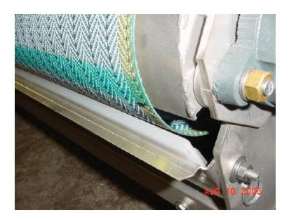
This picture shows the discharge end roller Fender installed.
