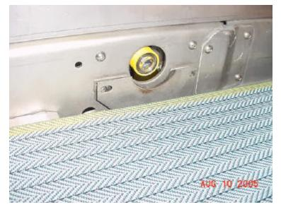
This picture shows the scraper mounting hardware in place. The bolt and nut as a pivot point and the pin as the angle set. The bolt can be used to lock the position of the scraper if the pin is not used.
