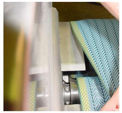
This picture shows the discharge end roller fender installed on a press with an extended conveyor. Note the photo eye is not visible in this picture due to the elongated belt.
