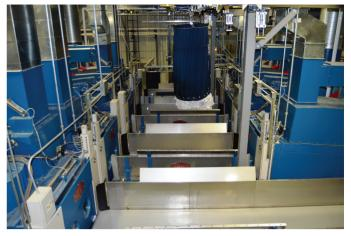
PRESS-TO-DRYER TRANSPORT: The E-Tech rail system is seen here delivering washed and extracted linen to the dryers
