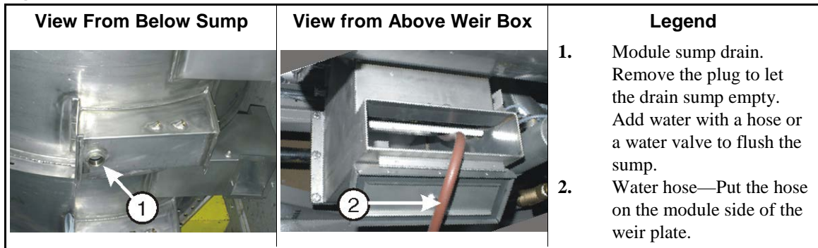
Figure 29: Module Sump Drain and Weir Box. These are examples. Your machine can look different.
