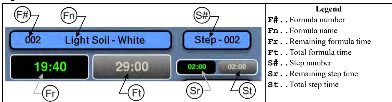
Figure 10. The Names and the Timers Area
