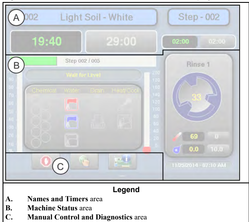
Figure 9. The Three Information Areas of the Run Display
